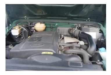
Step 2: Remove the pipes from the EGR valve
