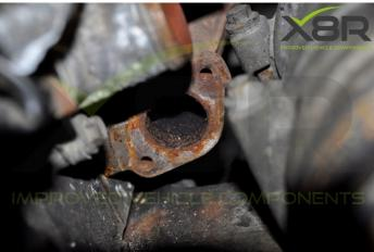
Step 7: Blank off the vacuum solenoid
